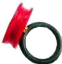
C) Place the rubber ring 24 x 5 mm. Adjust the brass tube to protrude 2 mm on each side.
