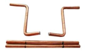
It is very important that the folded parts are carried out exactly in the middle of the brand to fit well.
